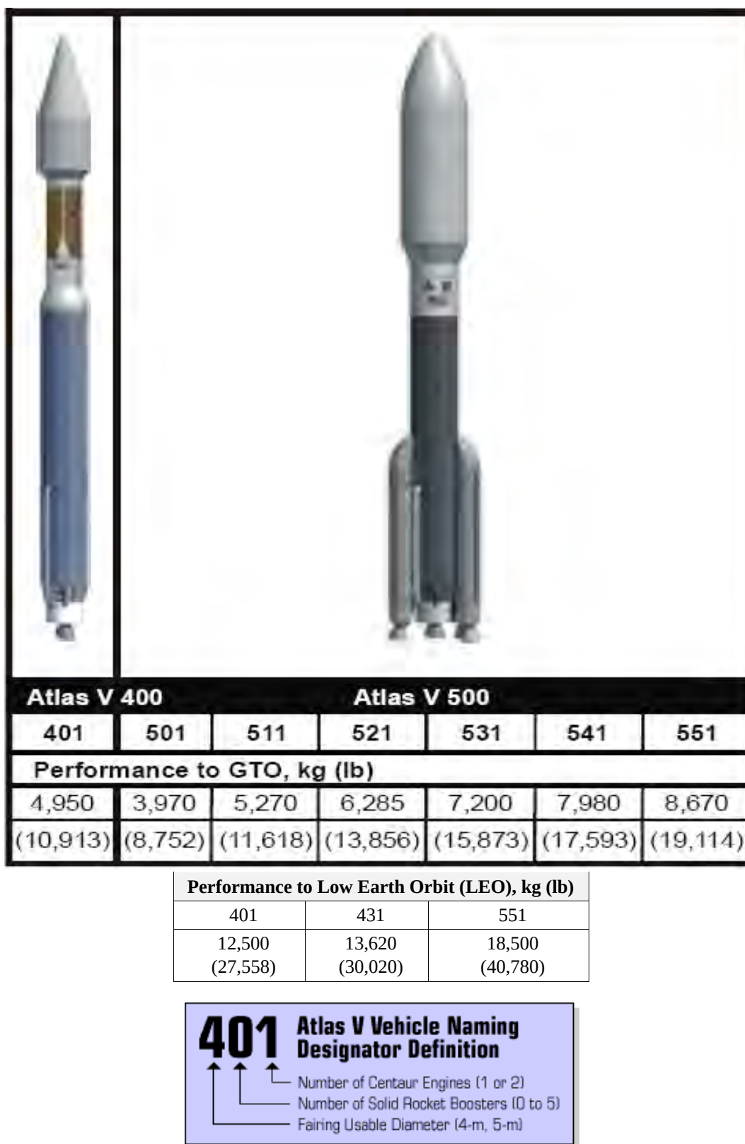
Figure 2–3. Atlas V Family of Launch Vehicles and Payload Mass that can be Lifted to Specific Orbits
