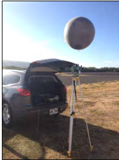
Figure 3: 30 gram Pilot Balloon and Observation Equipment
