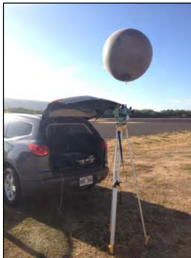
Figure 3: 30 gram Pilot Balloon and Observation Equipment
