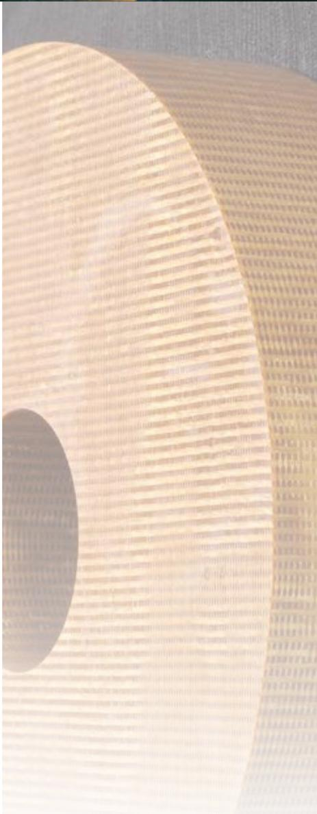
*NASA's 3-Dimensional Multifunctional Ablative Thermal (3D-MAT) Protection System project designed and developed a game changing woven thermal protection system (TPS) technology tailored to the needs of the Orion Multi-Purpose Crew Vehicle (MPCV) compression pad for the lunar return mission, EM-1, and beyond. (NASA)*
