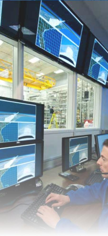
*James Peckham, an nLogic Inc. test engineer supporting the Stages Office at the Marshall Center, runs an avionics flight simulation to see how SLS will perform during launch. (NASA/Boeing)*
