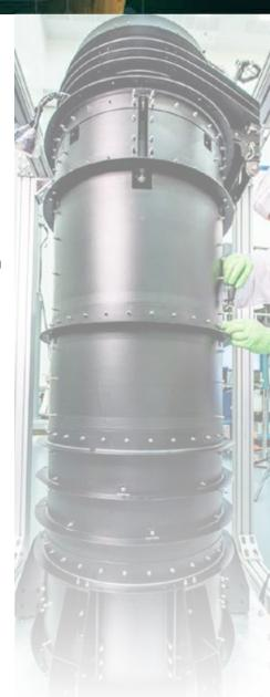
Recently, engineers at Northrop Grumman Corporation in Redondo Beach, California were testing the Deployable Tower Assembly (DTA) for the James Webb Space Telescope (JWST) to ensure it worked properly. (NASA/Northrop Grumman)
