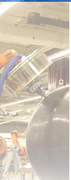
A robot places composite fibers on the tank's inner wall structure. Engineers at Boeing Research & Technology formed the composite cryogenic tank using automated fiber placement at the Boeing Developmental Center in Tukwila, Washington. (NASA)
