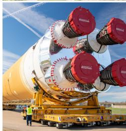
MAF manufactures and assembles the largest rocket stage NASA has ever constructed: the Artemis missions' Space Launch System (SLS) core stage—the world's most powerful rocket that will send the Orion spacecraft, astronauts and supplies on bold exploration missions to the Moon and beyond.
