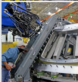
Orion's large structures and composites are also being manufactured at Michoud. These structures include the Orion crew module pressure vessel and its underlying framework, designed to ensure a sealed life support environment. Fabrication and of Orion's launch abort system also occurs at MAF.
