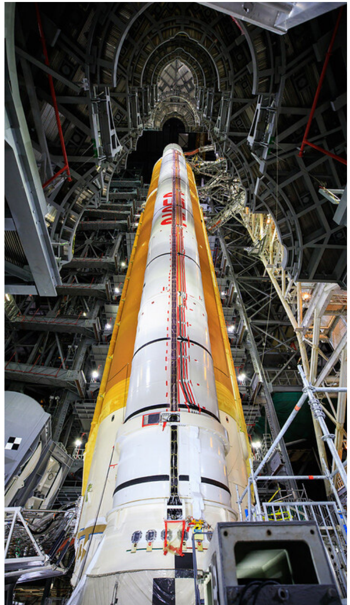
Artemis I boosters and core stage structurally mated in the Vehicle Assembly Building at Kennedy Space Center in Florida. (side view)
