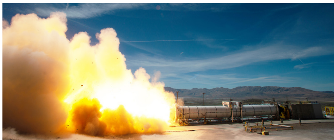
Boosters undergo hot fire tests to evaluate materials and processes for future missions.
