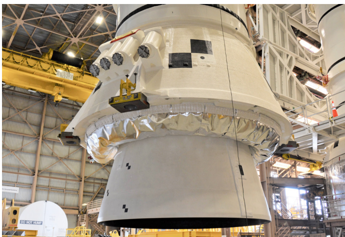
Artemis I booster aft assembly stacked on the mobile launcher in the Vehicle Assembly Building at Kennedy.
