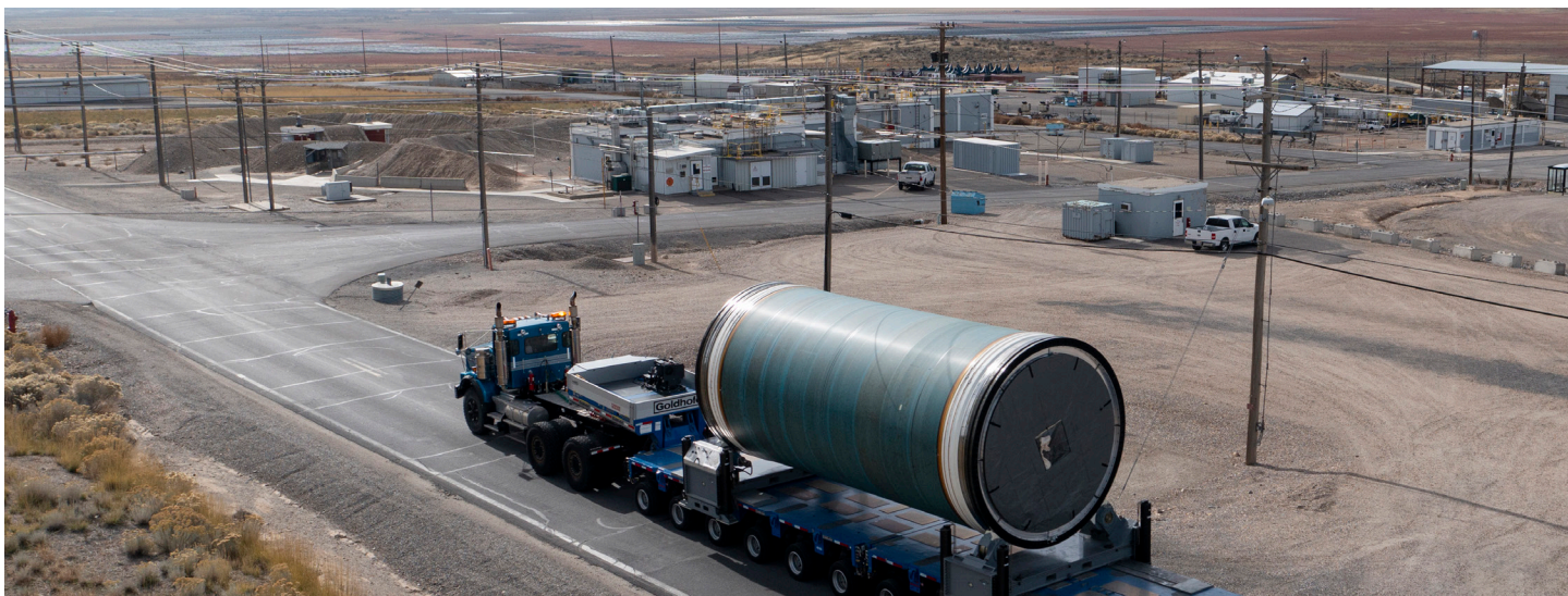
A booster obsolescence and life extension (BOLE) motor segment being transported to final assembly at Northrop Grumman in Utah.
