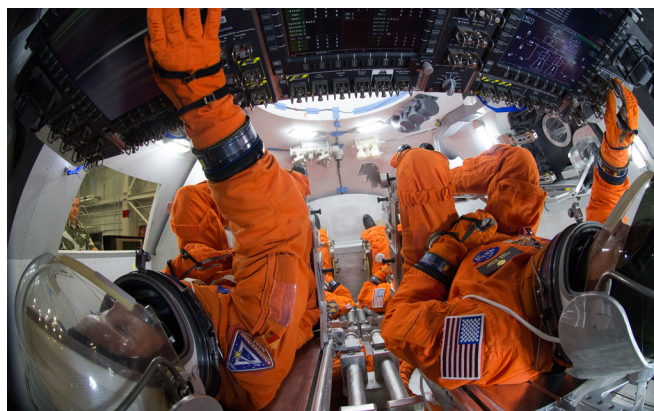
Spacesuit engineers demonstrate how four crewmembers would be arranged for launch inside the Orion spacecraft, using a mockup of the vehicle at Johnson Space Center.
