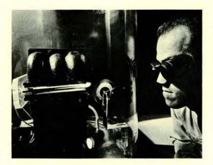
A miniature laboratory ionpropulsion model, operating at near vacuum conditions, produces thrust which is detected by the small wheel behind the jet. An ion jet is produced when charged particles are formed in an electric discharge between two electrodes, and are accelerated by a magnetic field. An ionpropulsion unit serving as a low thrust engine may be useful in flight at extreme altitudes. However, many problems must be solved before it will be practical.
