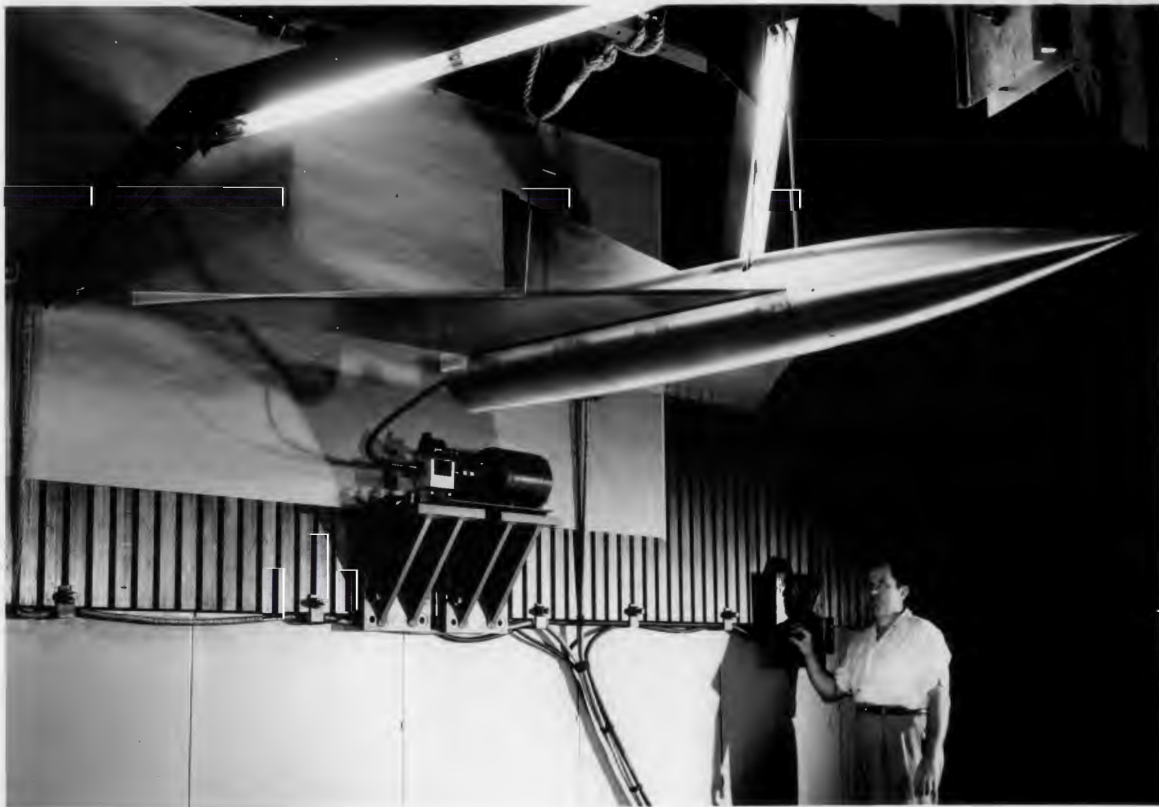
Demonstration of the Effect of Heating on the Vibrational Characteristics of a Model
