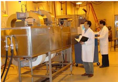
Pressure Assisted Thermal Sterilization (PATS) and Microwave Assisted Thermal Sterilization (MATS)
