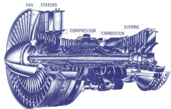
Typical high bypass ratio engine
