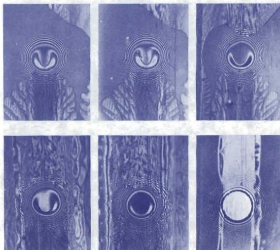
Photomicrograph of progressive lubricant starvation of bearing
