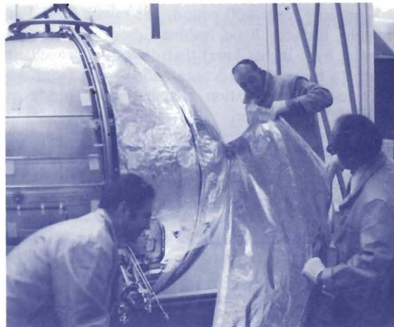
Insulating a liquid hydrogen tank
