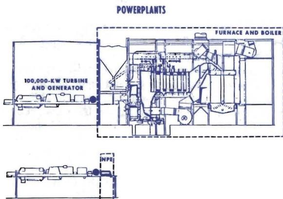
Size comparison of coal fired steam plant for electric power generation with one using rocket type combustor
