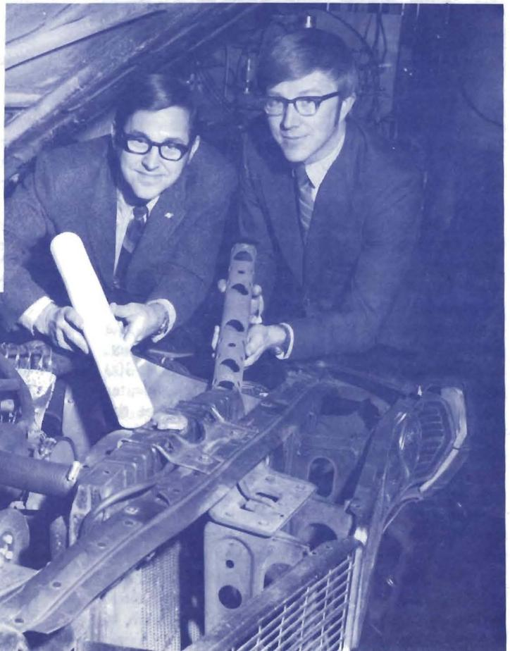
Experimental thermal reactor for automobile pollution control
