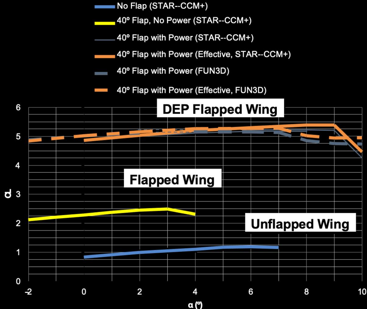
*DEP can provide highly coupled aero-propulsive integration to highlift systems to provide significant low speed lift augmentation, without the typical problems such as high pitching moments associated with circulation augmentation due to aft loading of the wing airfoil (or additional noise sources).*
