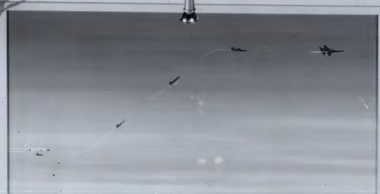
THE X-15 "L" JETTISONING ITS EXTERNAL PROPELLANT TANKS AFTER THEY ARE EMPTY, ACCELERATES TO SUSTAINED HIGH SPEED TO FLIGHT TEST VARIOUS AIR-BREATHING PROPULSION SYSTEMS.
