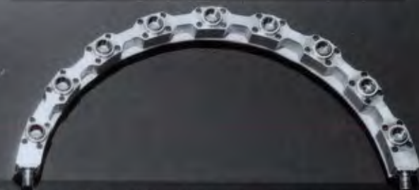
IMPEDANCE RING - MEASURES VHF ANTENNA CHARACTERISTICS
