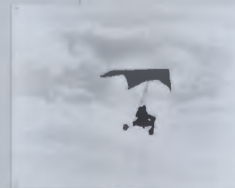
DURING GLIDE FLIGHT THE PARASEV HAS A FORWARD SPEED OF ABOUT 70 MILES PER HOUR. THE DESCENT FROM 10000 FEET TAKES ABOUT 3 MINUTES.
