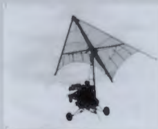
THE PARASEV IS CONTROLLED BY TILTING THE FLEXIBLE WING FROM SIDE TO SIDE AND/OR UP AND DOWN.
