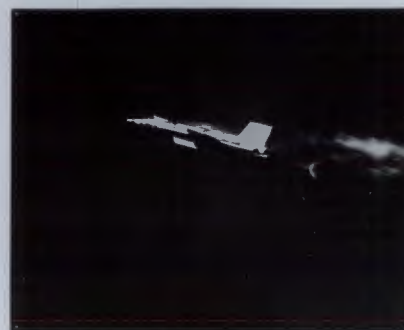
SHOCK WAVES FORM IN THE EXHAUST PLUME OF THE ROCKET ENGINE AS THE X-15 BEGINS TO CLIMB UPWARD.
