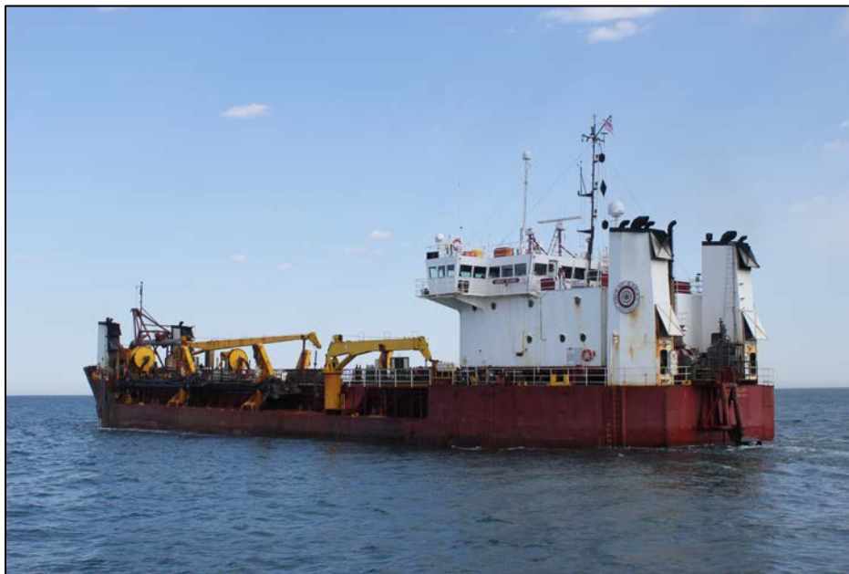
Figure 2-6: Trailing Suction Hopper Dredge with Dragarms Raised
