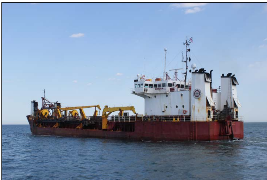
Figure 2-6: Trailing Suction Hopper Dredge with Dragarms Raised
