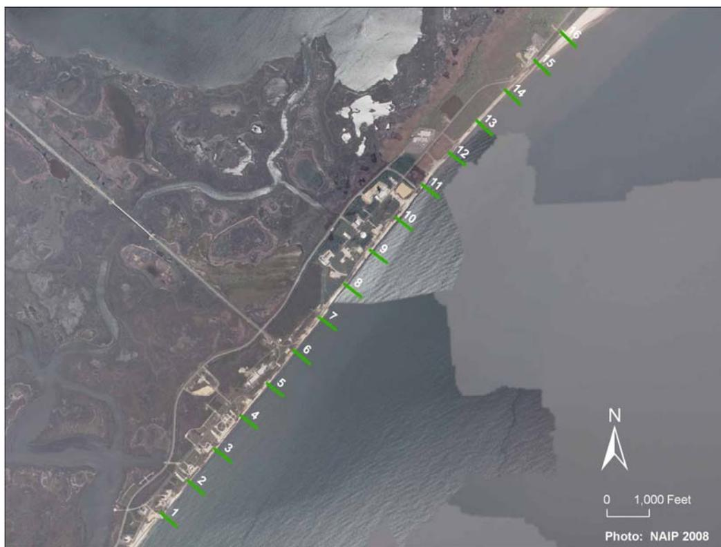
Figure 3-27. Locations of analysis cross-sections for seawall repair to +12 and +14 ft.
