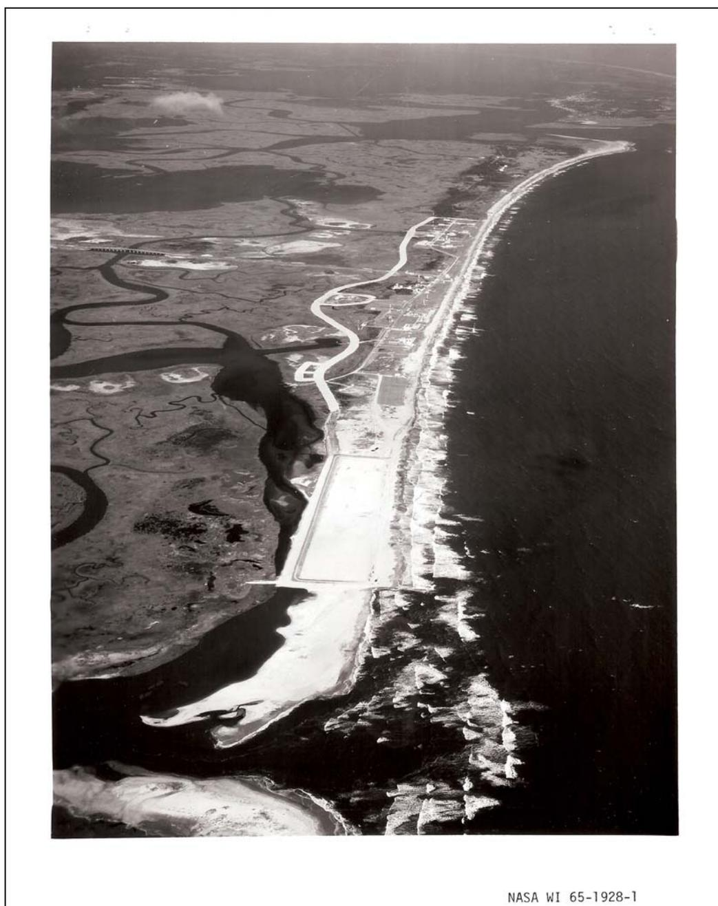
Figure 2-8. Mechanically filled section of the south end of Wallops Island following an Ash Wednesday Storm breach.
