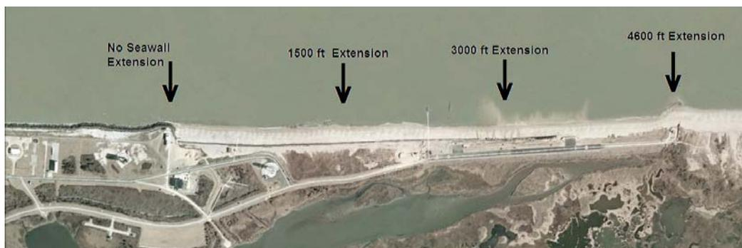
Figure 10-1. Potential seawall extensions modeled in this study.
