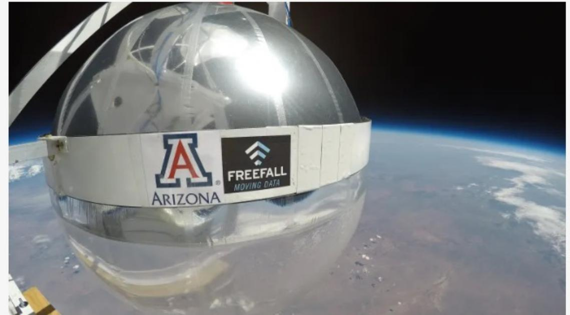
FreeFall Tests Spherical Antennas at 159,000 feet on NASA's 60 million cubic foot stratospheric balloon.
