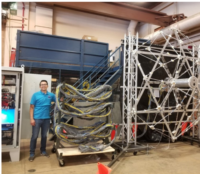
Figure 1. Overall view of the MPA, cable bundle, and data acquisition cabinet.
