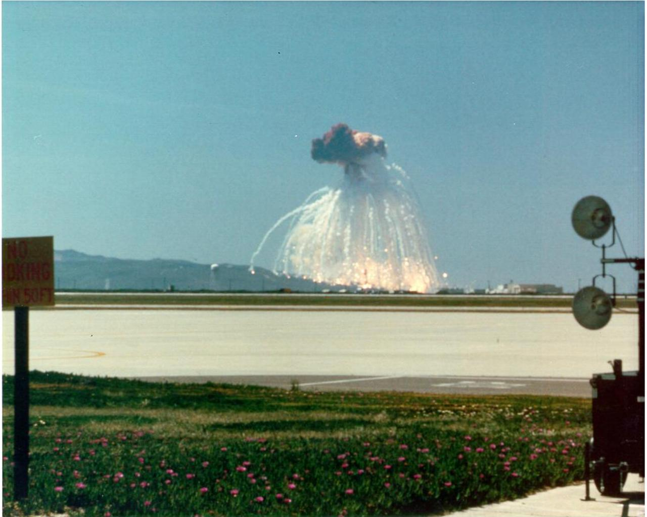
**Figure 5-9. Solid Propellant Conflagration Cloud (White) and Liquid Hypergol Deflagration Cloud (Red) Formed When the Titan 34D-9 Vehicle Exploded at Vandenberg AFB.**
