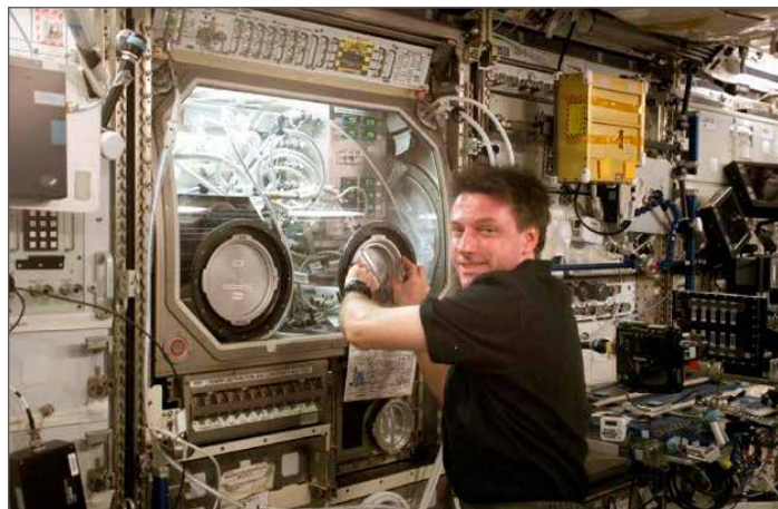
Expedition 8 Commander and Science Officer Michael Foale conducts an inspection of the Microgravity Science Glovebox.
