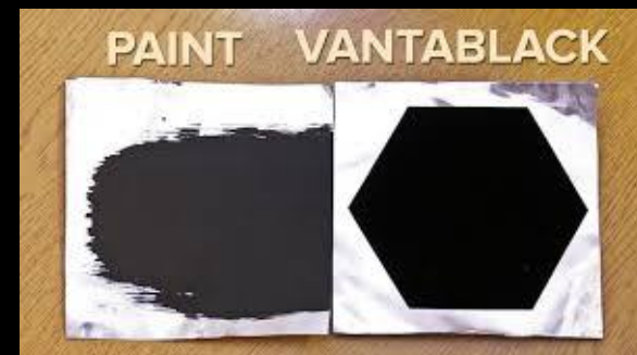
Ultra-black surface coatings can potentially relax requirement on edge sharpness
