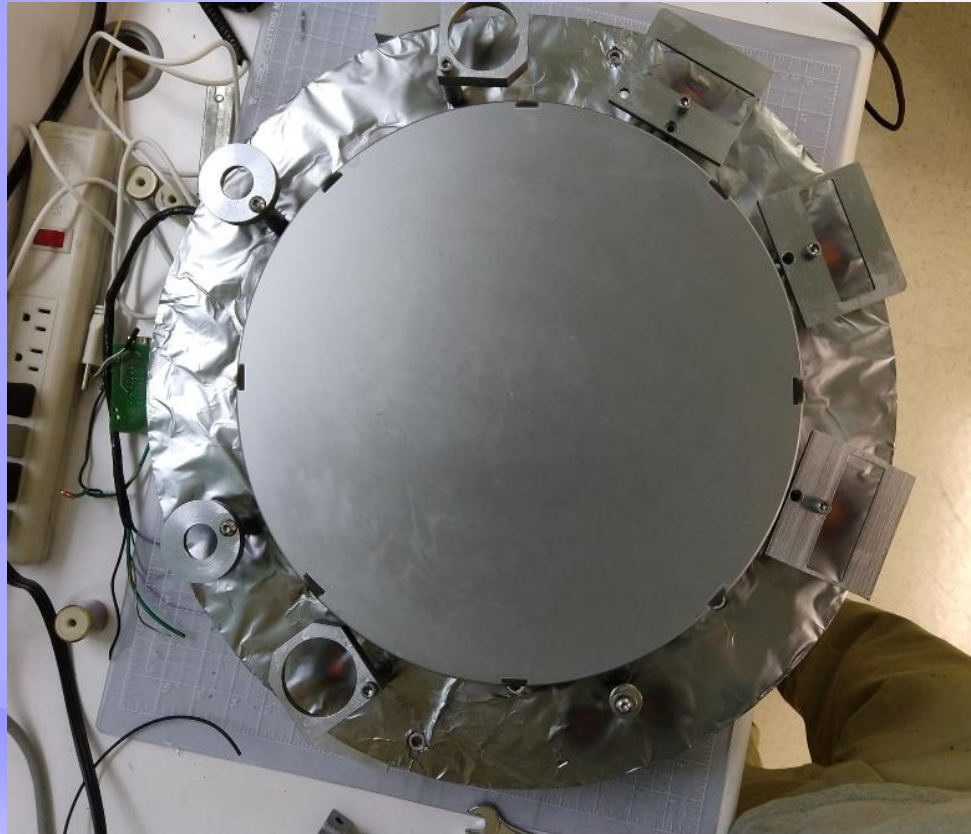
Mirror substrate after silicon cladding by ZeCoat (14" dia.).
