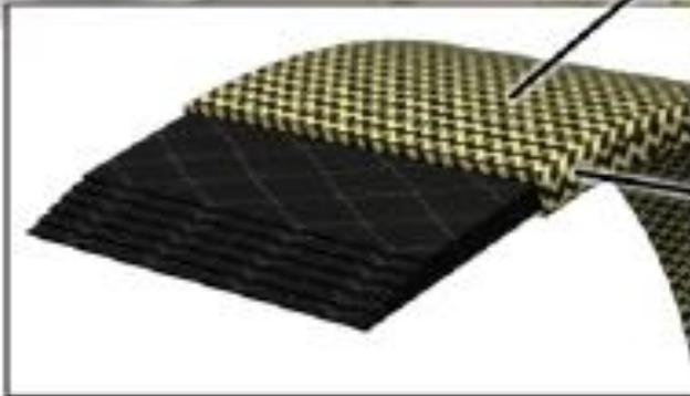
Dimensionally-Stable Structural Space Cable (DS3 Cable) proposed for the Starshade spoke
