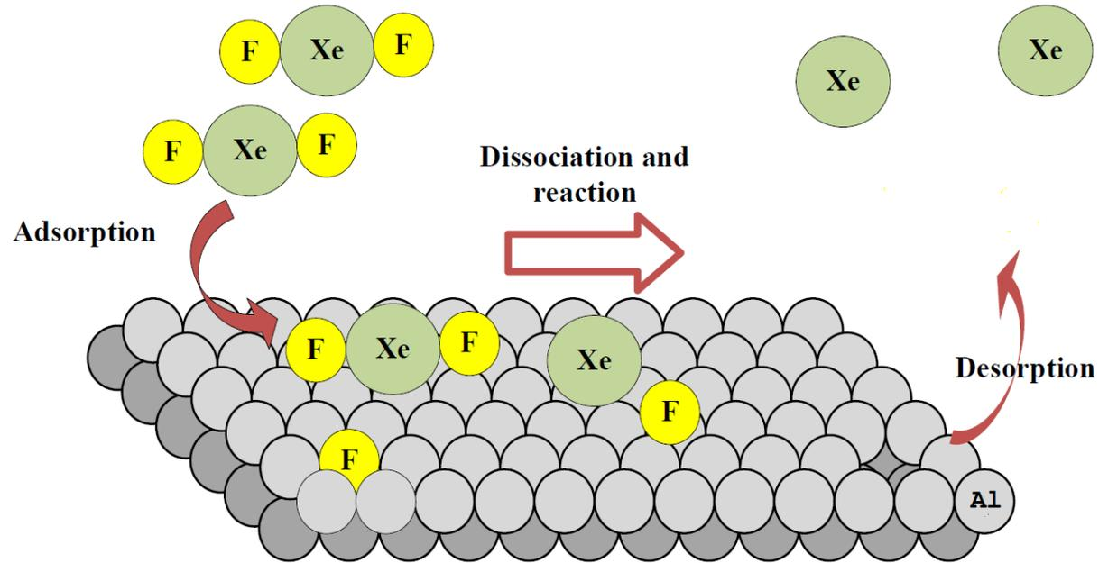
XeF<sub>2</sub> is a dry-vacuum based method of reaction and requires no plasma or other activation minimizing damage to substrate.
