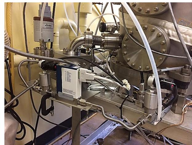
XeF<sub>2</sub> Gas feed components capable of continuous flow or pulsed flow.
