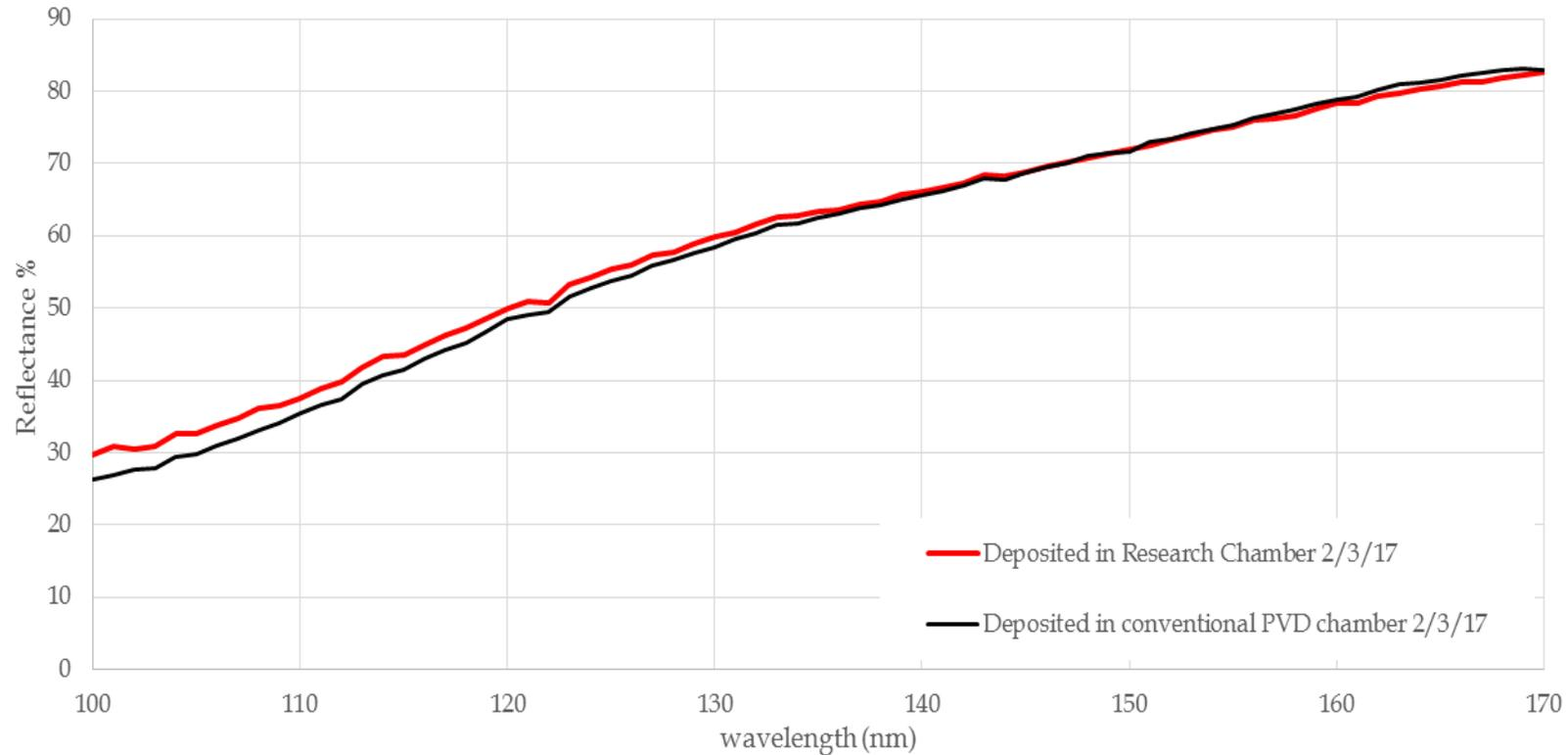
Aluminum coating thickness: 50-70nm @ 130-160 A/Sec
