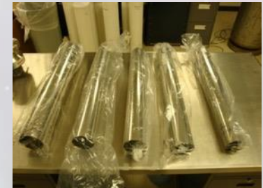
8. Separate optic from mandrel – reuse mandrel for next shell
