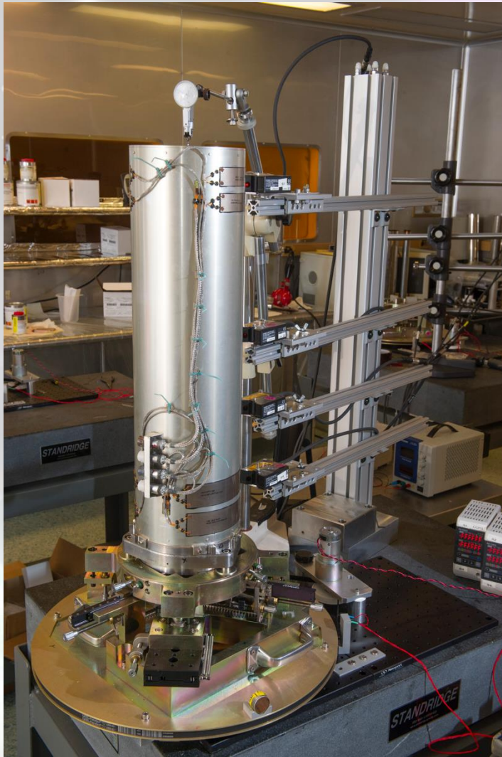
ART-XC shells supported from 3 points during the alignment and bonding process
