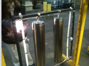
2. Chemical clean and activation & Electroless Nickel (EN) plate
