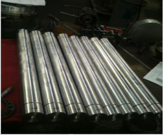
1. CNC machine, mandrel formation from Al Bar
