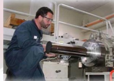
3. Precision turn to sub-micron figure accuracy
