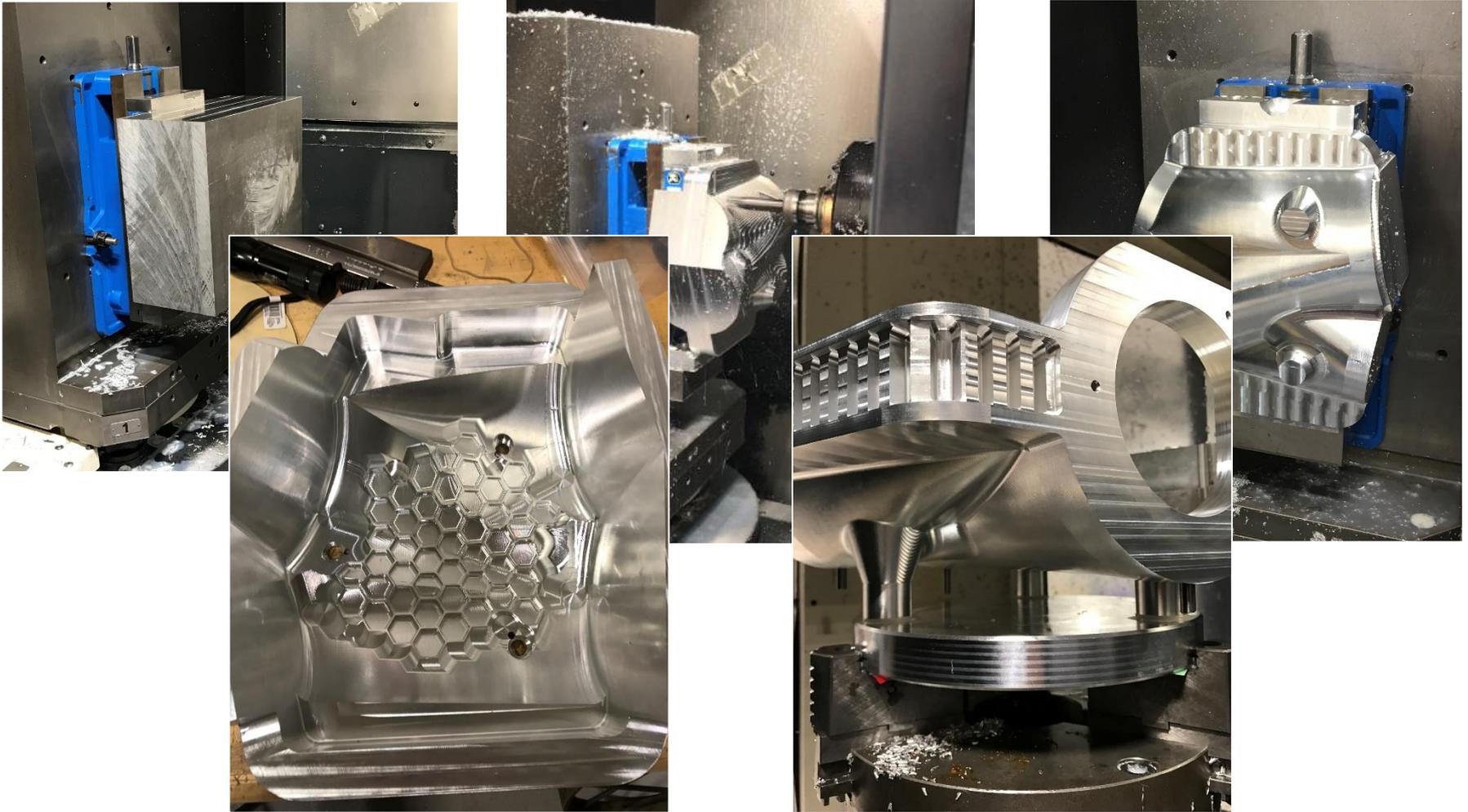
Optics were designed and fabricated with fiducials for prescription orientation, assembly metrology, and mounting features in one manufacturing setup
