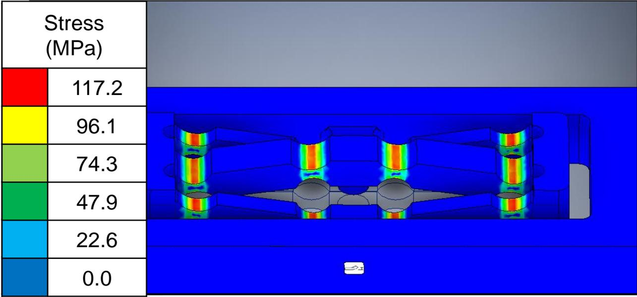
Finite Element Analysis of Flexure
