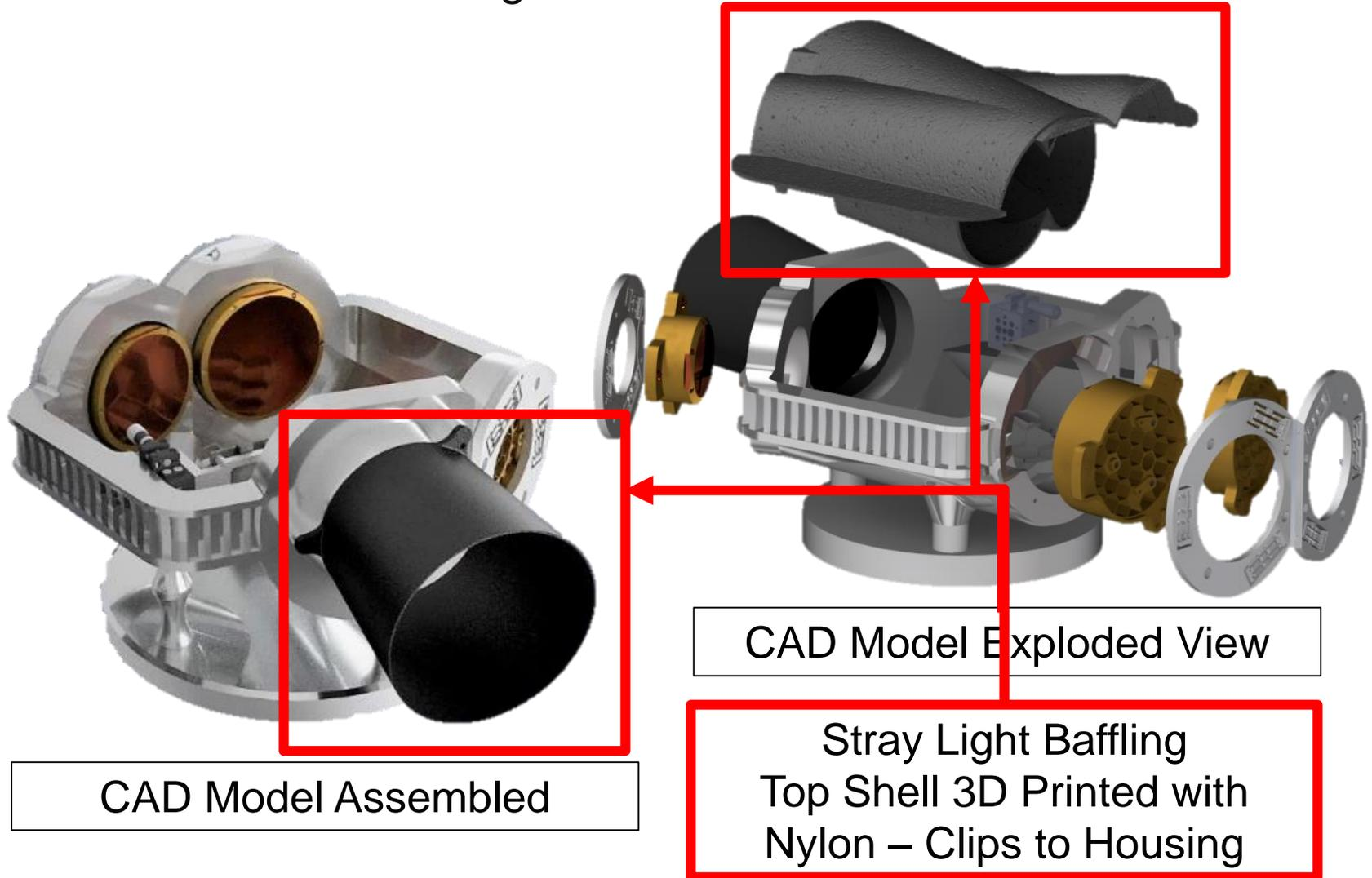
The assembly requires no special tooling, gage blocks or instructions. It can be assembled and imaged in less than 10 minutes.
