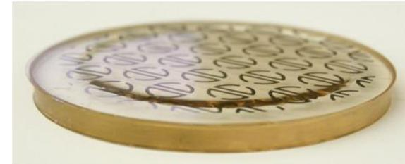
*Ghz antenna field for frequency selective surface under coverlayer, printed on VBX film with VHX silver nanoparticle ink*
