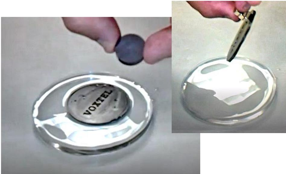
*Floating polymer moving to magnet, lifted by magnet*
