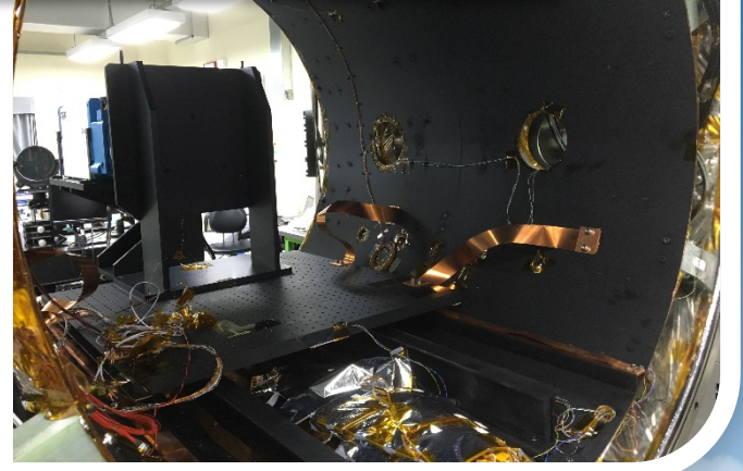
WFE measurement while changing temperatures (+20C, -10C and -40C)
