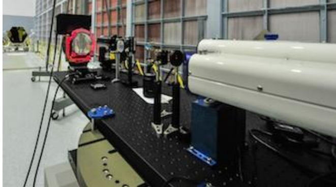
This photograph shows all the optical elements in the test setup including the HSI, CGH (framed in red), and test mirror (hexagonal mirror on the far left).
