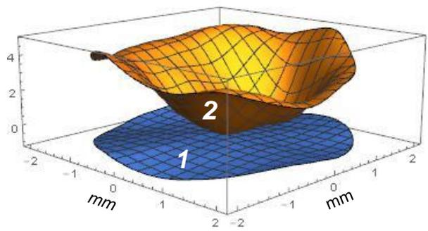
The wavefront of the reference wave reflected by a plane mirror (1) and DM2 mirror (2). The scale of the vertical axis is equal to the reference wave wavelength ( $\lambda = 625 \text{ nm}$ ).
