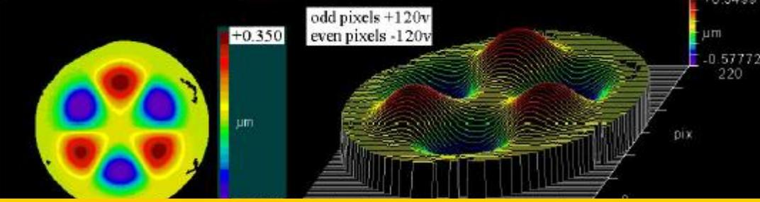
**ARL 7-pocket 49-channel DM with Controller**
