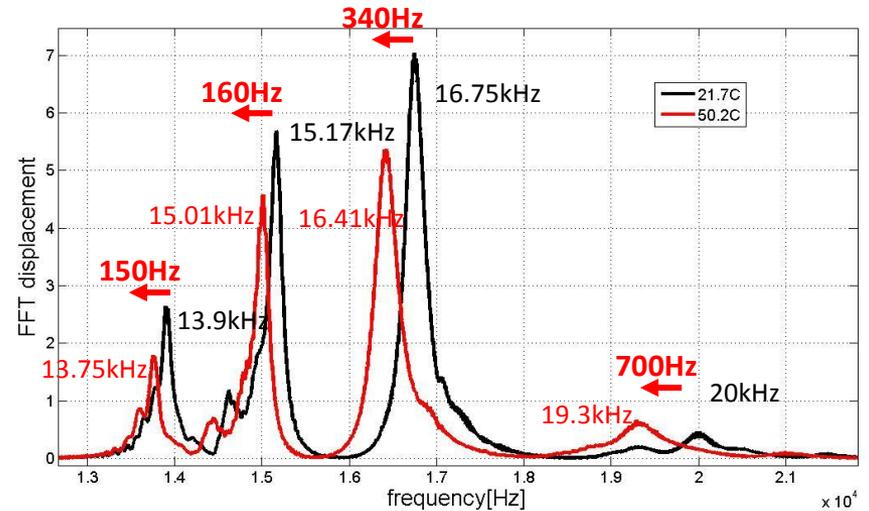
Temperature dependence of channel #5 resonant modes (black curves: 21.7C, red curves: 50.2C). PZTs parallel excitation at 10V: (a) 2-3.1kHz sweep frequency excitation; (b) 13-22kHz sweep frequency excitation.
