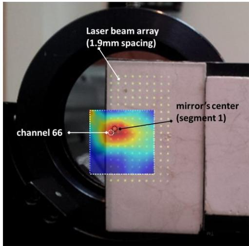
2D displacement FFT at 300Hz superimposed on the mirror's image
