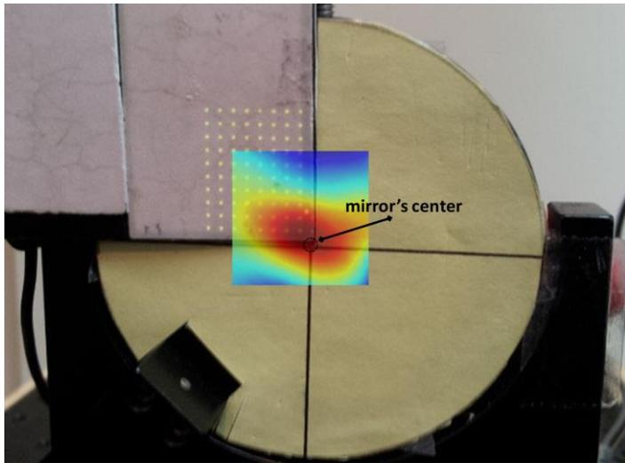
2D displacement FFT map at 10kHz superimposed on the mirror's image
