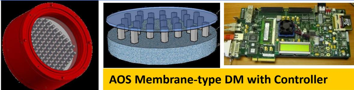
**AOS Membrane-type DM with Controller**
