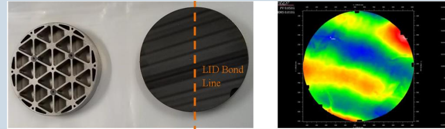
Be-38Al / LID Bonding / Electroless Nickel Plating (CTE Matching) / SPDT- Polished
