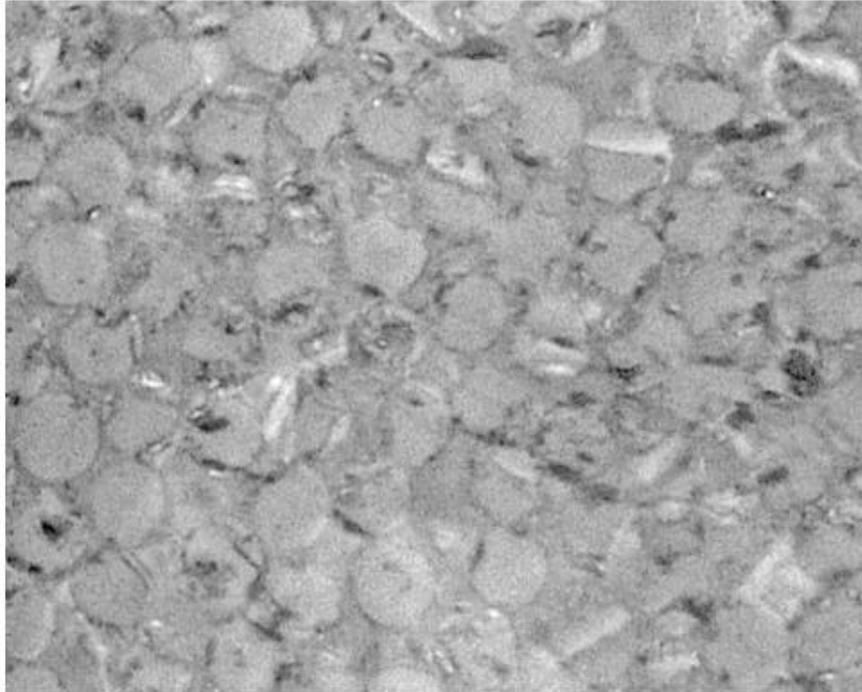
Panel cross section at 3500X after five infusion cycles
