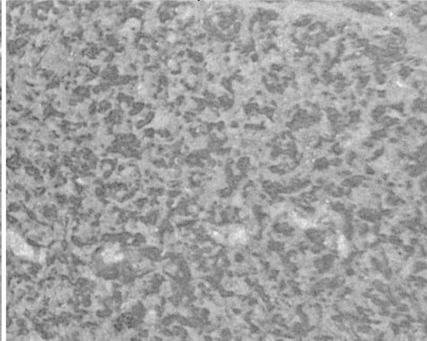
Note that the individual quartz fibers are still round and have definition on the left. After the infusion process, the fibers have lost their round shape and definition, indicating that conversion is happening
