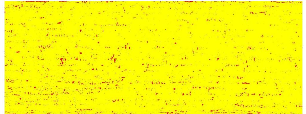
Porosity (shown in red) of cross section of DSS-19 after infusion trials. Porosity is at 2.09%
