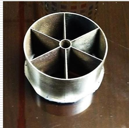
Laser sintered titanium baffle
