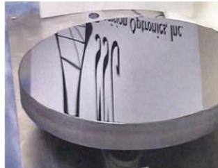
Photo of Silicon Coated SiC Aspl Finished Optic
