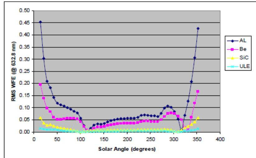
RMS Wavefront Errors (primary mirror only) as a function of solar loading angle for different primary mirror materials
