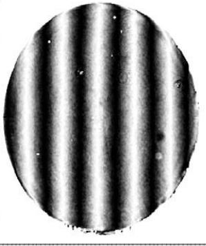
Fig. 6 Interferogram from Silicon Coated SiC Aspheric Optic (0.012  $\lambda$  RMS)
