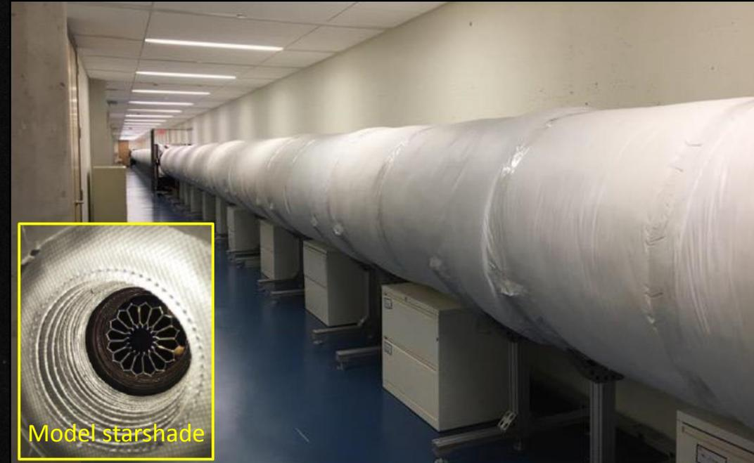
S5's starshade model validation testbed at Princeton.
