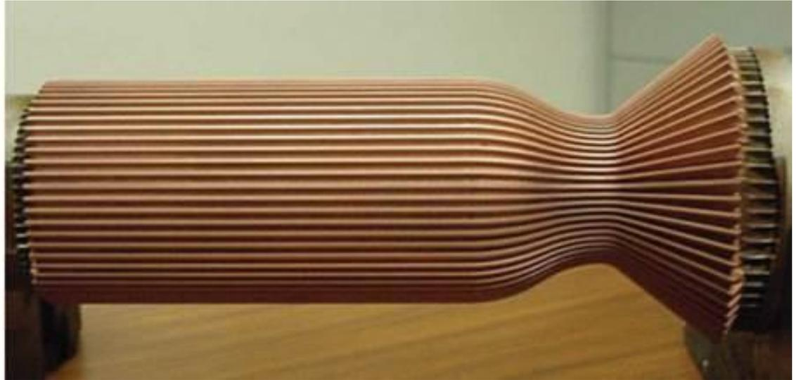
2015 phase II SBIR: Low Cost Manufacture of nozzles and combustors for channel wall liquid rocket engines.
