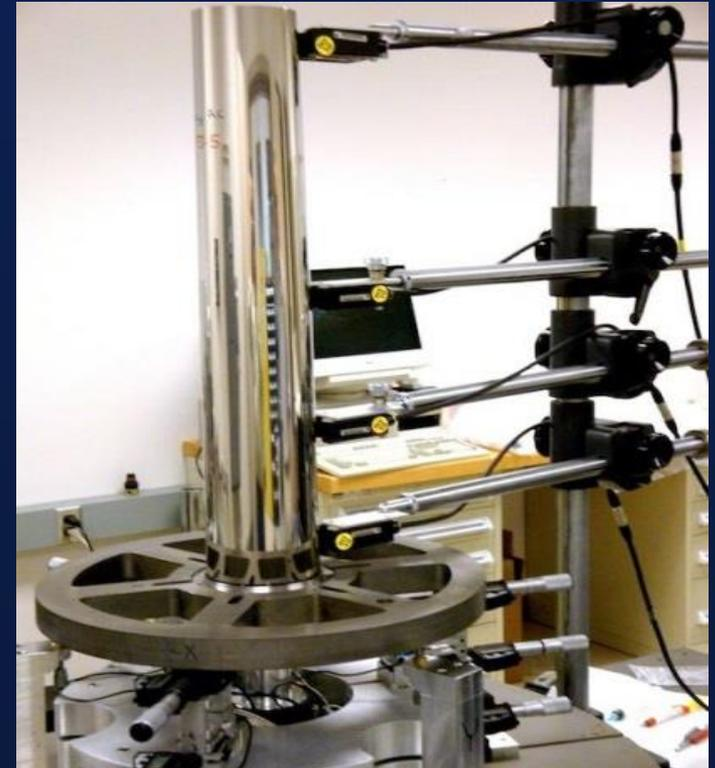
The x-ray optics module alignment station used for the FOXSI project
