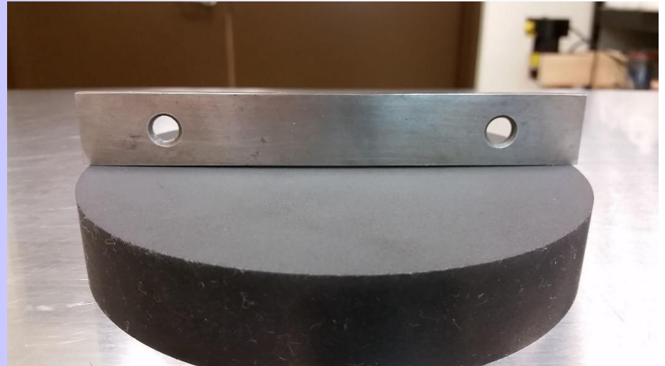
Uncoated ceramic mirror blank with F2 curvature ground into surface
