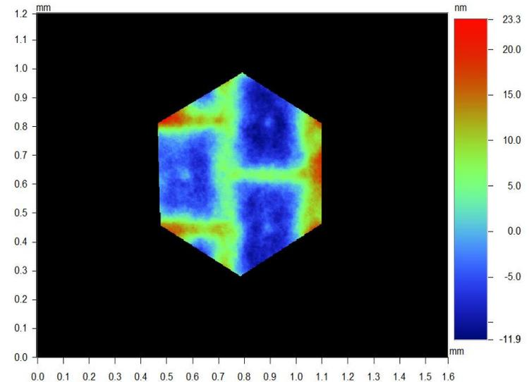
Individual segment 7 nm RMS over 760 $\mu\text{m}$
