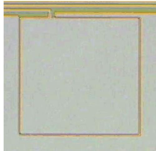
2μm spaced electrode optical images 10 minutes apart with 275V applied
