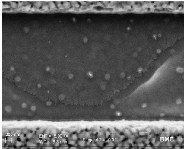
SEM of foreign material seen in the 3um electrode cuts of fabrication material leading to the reduced yield.
