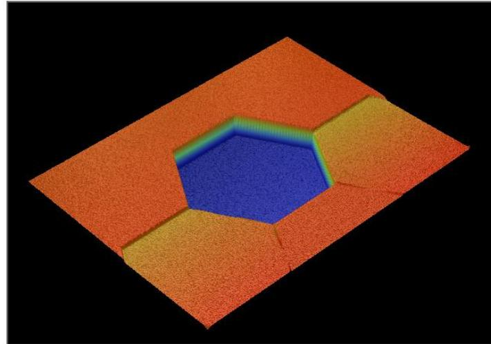
Stiff actuators results in low influence function, allowing for steeper tilt.
