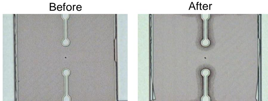
Damage seen after 11 million flexure cycles to 295V
