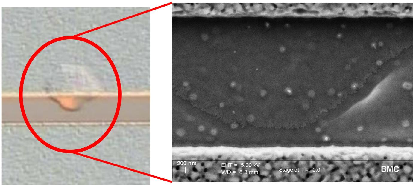
Optical Image and SEM of foreign material seen in the 3um electrode cuts of fabrication material leading to the reduced yield.
