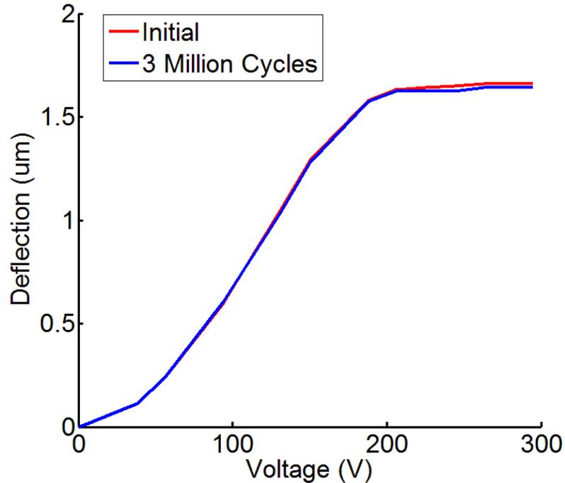
Deflection versus voltage. Initial, after cycling 3 million times above critical voltage (295V).
