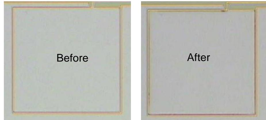
Damage seen on 3μm spaced electrode held for 1 hour at 275V
