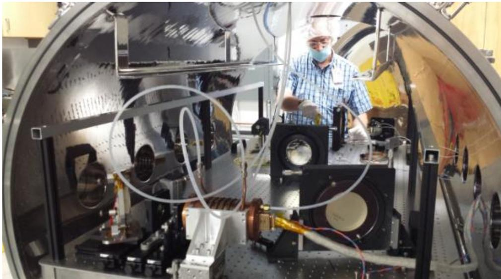
Vacuum Surface Gauge (above) in development to characterize DM actuator stroke accuracy and stability to ~30 picometers
