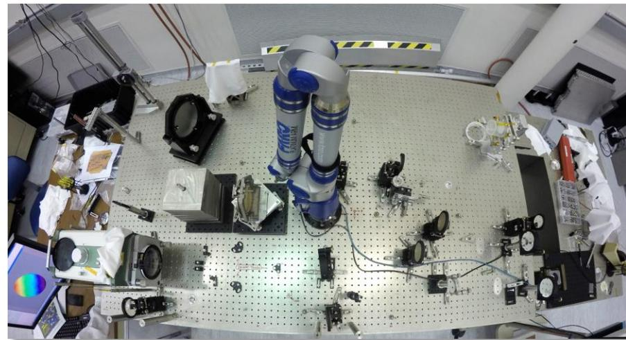
Northrop Grumman Xinetics electrostrictive Deformable Mirrors used in HCIT since 2003 ( $10^{-9}$  raw contrast demonstrated)
