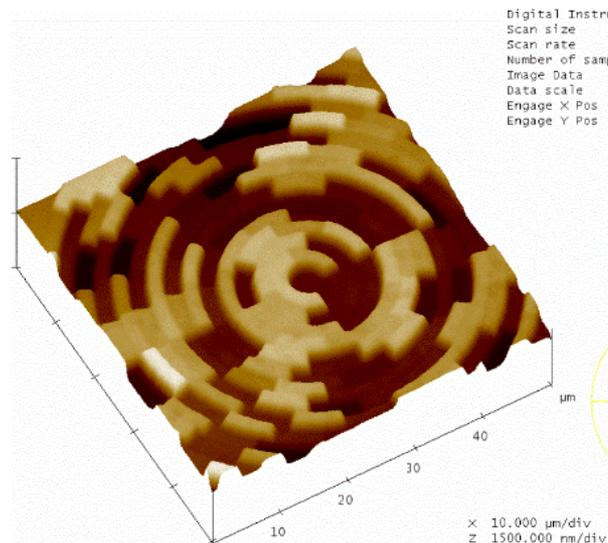
PIAACMC mask image with an atomic force microscope
