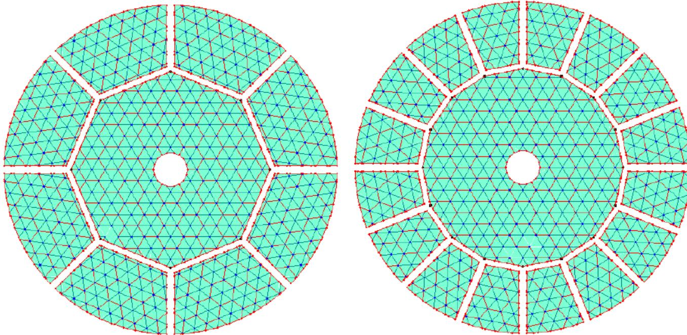
One option for limited shroud diameter is to have as large a central monolith as possible, with deployable petals. This provides a better diffraction pattern than uniform segment patterns, as well as more mission flexibility.
