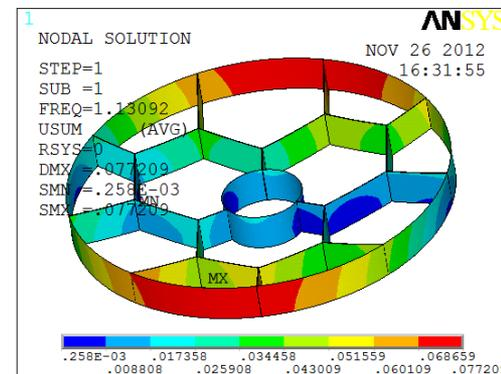
Internal Stress: 4 m dia with 6 support pads
