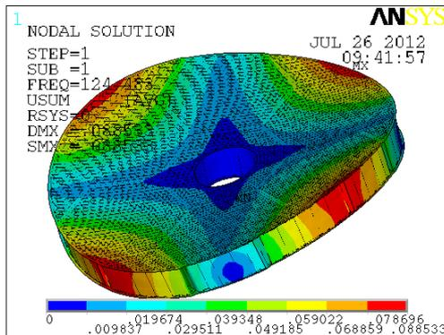
Free-Free 1<sup>st</sup> Mode: 4 m dia 40 cm thick substrate
