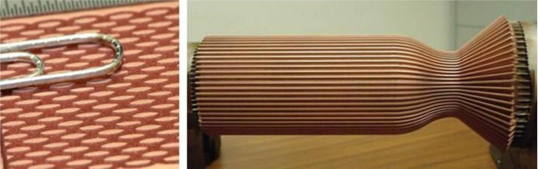
2014 phase II SBIR: Milling rocket engine channel wall for SLS's Low Cost Manufacture Expendable SSME for NASA/Aerojet.
