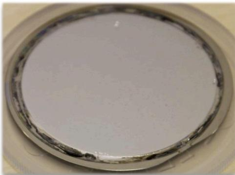
Process development using NiCo plated silicon wafers (due to mandrel availability), continued testing on conical mandrels to evaluate X-ray performance
