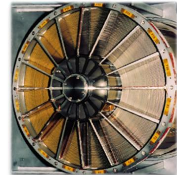
Current State of the Art X-ray observatory (XMM Newton) utilizing 58 nested reflector shells; largest reflector 70cm diameter.
