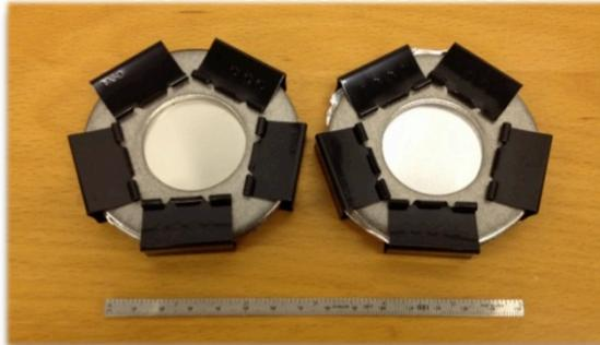
Evaluate potential particle damage using nickel and aluminum foil
