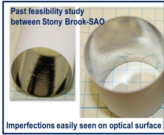
Successfully released reflector coating from the mandrel
