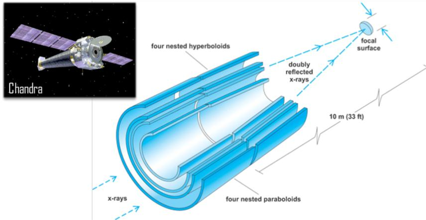
Chandra X-ray observatory utilizing 4 nested zerodur optics with the outer shell measuring 1.2 meters in diameter.
