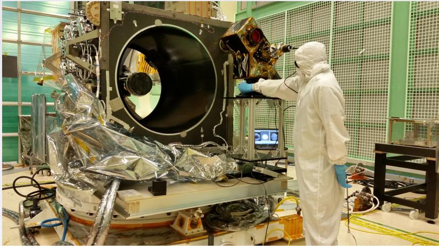
Ambient Testing of Advanced Technology Large-Aperture Space Telescope (ATLAST) Instrument Reflector Telescope Assembly
