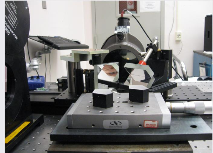
2-Axis autocollimator used to measure mirror deviation
