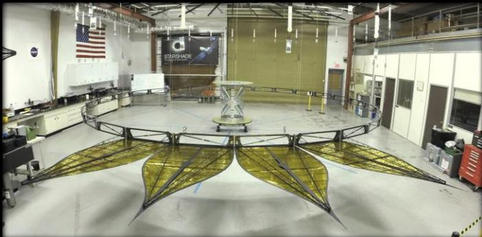
Half-scale inner disk testbed (JPL)
