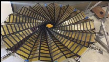
1/10-scale opaque membrane testbed (JPL)
