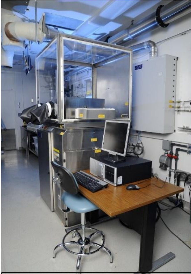
ALD coating system at JPL; gas feedthroughs and process controls enable \text{AlF}_3 and \text{MgF}_2 coatings development
