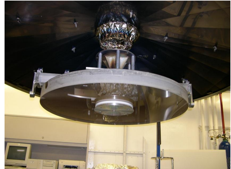
Chamber top Cover with mirror substrate installed
