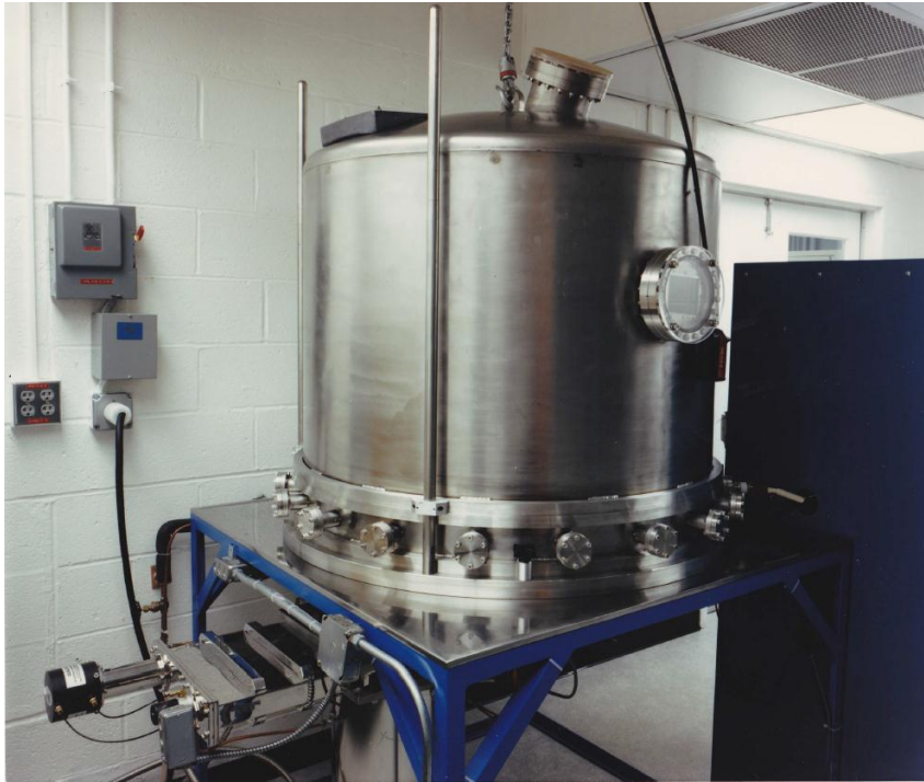
PVD coating chamber (1-meter)
