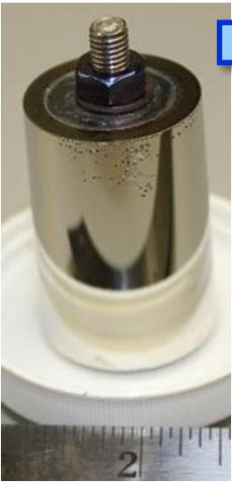
Successfully released reflector coating from the mandrel
