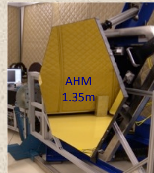
AHM SiC-based Segment Substrate
