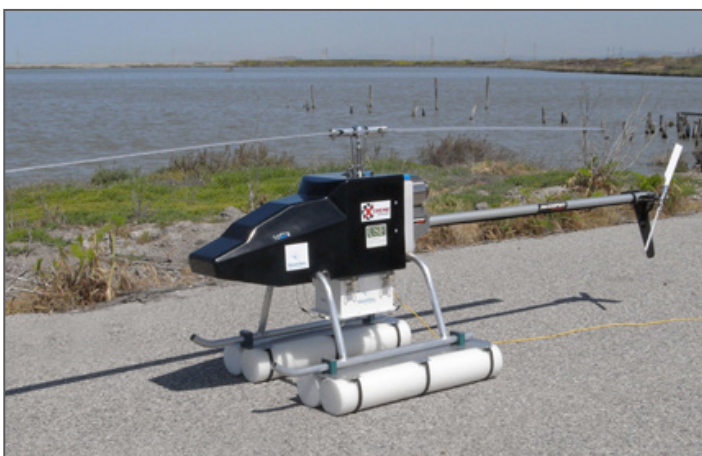
Vision-II during flight preparation with yellow cable serving to initialize NovaSol hyperspectral imaging system;
