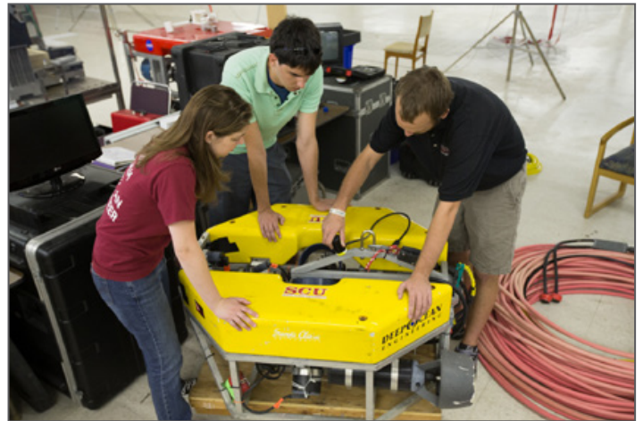
Santa Clara University students Anne Mahacek, Tom Hoye and Jimmy Erskine adjust a tracking beacon on the Triton underwater robot, which is being prepared for a mission in Lake Tahoe with scientists from the U.S. Geological Survey.
